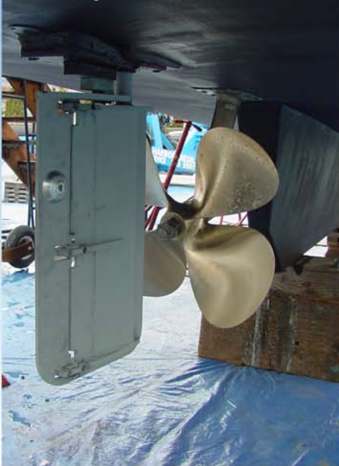
39 Mainship Trawler with Free Hanging Articulating Rudder
